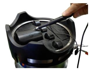
e Place the Sonar Head into a small bucket or tank and view the sonar returns.
