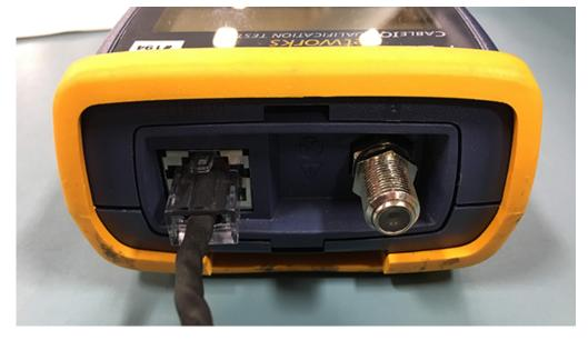
d Plug the other RJ45 connector on the test connector (on the other end of the spliced cable) into the RJ45 socket on the top of the cable tester.
