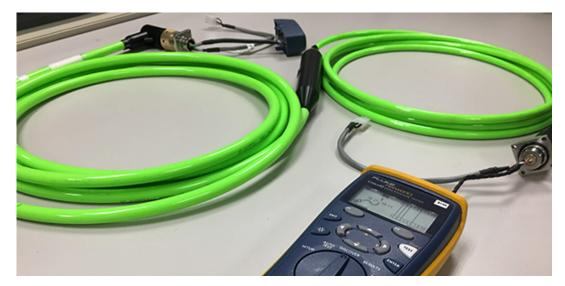
7 Test the electrical connections again using the cable tester and make sure that it is ready for use.
