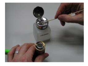
3 Inspect the o-ring for defects.
