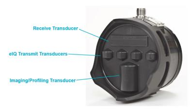
The Sonar Head includes transmit and receive transducers and the electronics to generate the transmit pulse and digitize the received signal. The sonar data is sent to the Sonar Processor using a standard Ethernet link.
