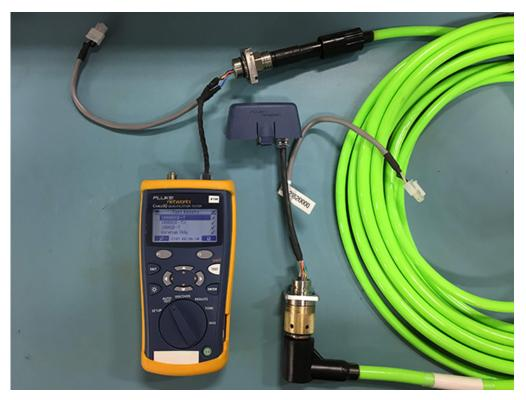
j Observe the test results and make sure that the *100BASE-TX* test passed.
