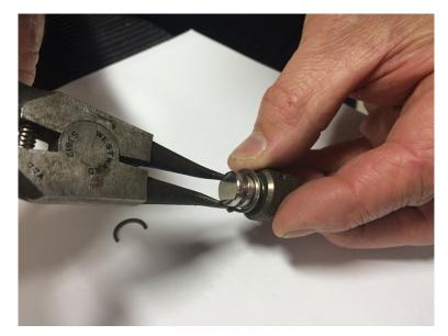
6 Slowly release pressure on the pliers and ensure that the retaining ring snaps into the notch.
