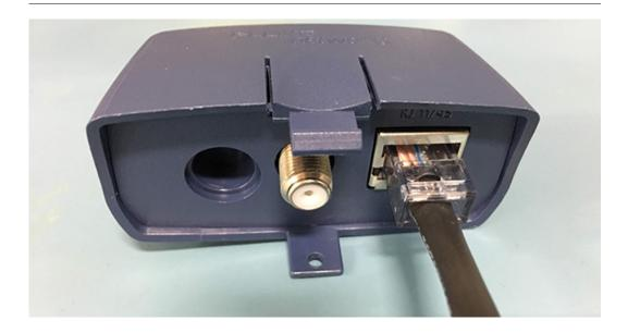
d Plug the other RJ45 connector on the test connector (on the other end of the spliced cable) into the RJ45 socket on the top of the cable tester.
