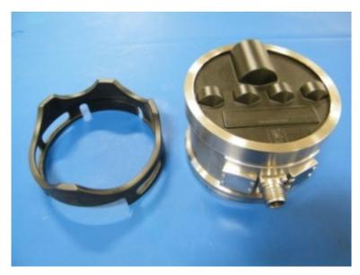
2 Place the Guard Ring on top of the Sonar Head, angled as shown.
