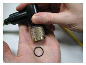
2 Clean the o-ring surface with Q-Tips and Isopropyl Alcohol. Ensure all dirt, hair, and debris is removed from the o-ring surface.
