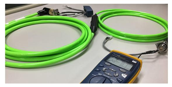
7 Test the electrical connections again using the cable tester and make sure that it is ready for use.
