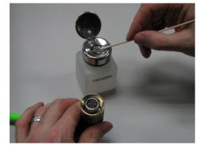
Inspect the o-ring for defects.Be sure to keep the o-ring free of dirt, hairs, or other contaminants.
