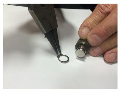
2 Insert the retaining-ring plier tips into the two holes in your replacement retaining ring.
