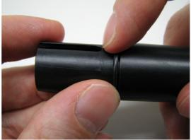
6 Using the DOIT, fit the o-ring back onto the Cable Connector Plug or Flanged Connector Receptacle.
