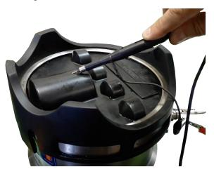
e Place the Sonar Head into a small bucket or tank and view the sonar returns.
