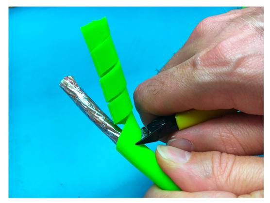
d Use the side cutters to cut off the sliced cable jacket.
