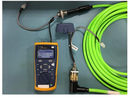
j Observe the test results and make sure that the *100BASE-TX* test passed.
