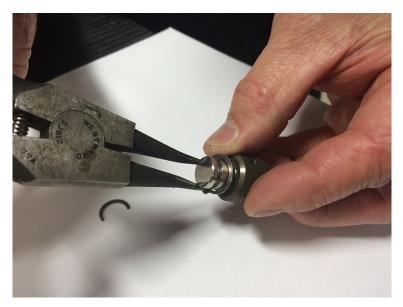
6 Slowly release pressure on the pliers and ensure that the retaining ring snaps into the notch.
