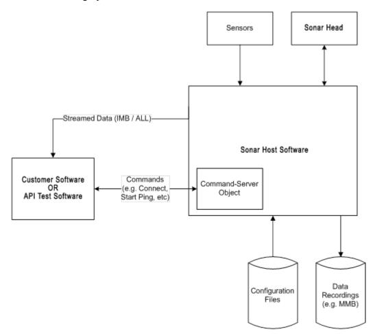
When the API is enabled, you can use your custom application (TCP client) to issue commands to the sonar. You can write API commands in XML format.
