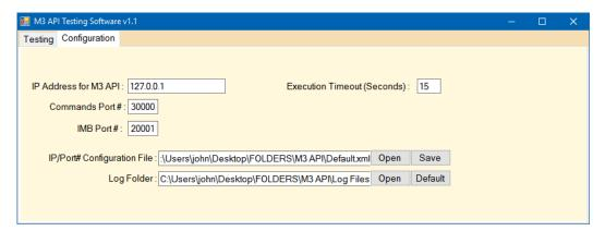
b If the M3 Sonar API is running on the same computer as the API Testing software, leave the IP Address as 127.0.0.1.
