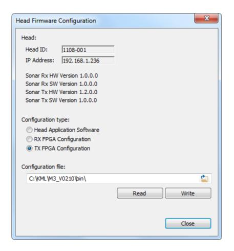
In addition to head application software, the Sonar Head has receive firmware (RX FPGA) and transmit firmware (TX FPGA). You can upgrade these by selecting the configuration type, browsing for the file, then clicking the **Write** button.
