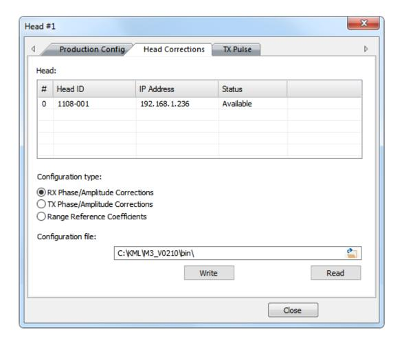
Use the **Head Corrections** page to write Phase/Amplitude Corrections or Range Reference Coefficients to the Sonar Head. This page is primarily intended for use by production test engineers.
