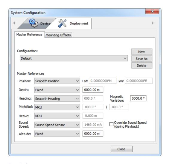
When using the Flexview for imaging, set up sensors for **Position** and **Heading** if you want to create GeoTiff files or create a real-time mosaic.
