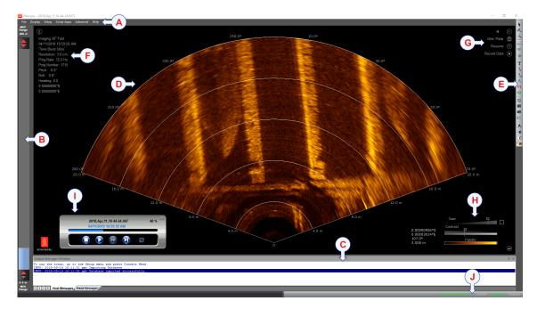
The presentation provides you with a lot of information. The sonar view presents sonar echo data. The menu system on the top gives you easy access to all the functionality offered by the Flexview software. The tool bar provides buttons for functions, filters, and sonar view overlays. The bottom **Output Messages** window and bottom status bar provide diagnostic messages.
