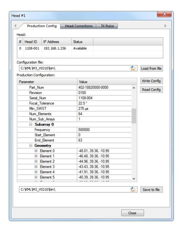
Use the **Production Config** page to view or change advanced Sonar Head parameters, such as the Serial Number or MAC Address. This page is primarily intended for use by production test engineers.
