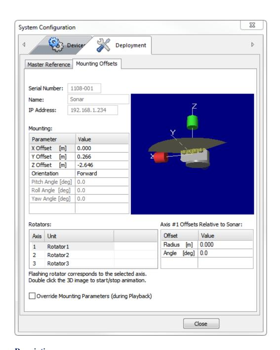
When you mount your Flexview Sonar Head on an ROV, you will need to specify where the Sonar Head is positioned in three-dimensional space relative to the GPS antenna.
