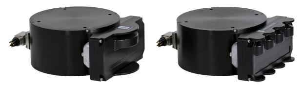
The removable transducer on the Flexview is the first of its kind, offering field replacement of a damaged transducer in the unlikely event of a catastrophic impact. This innovative design also allows for transducer configurations to be exchanged, depending on the job being performed. There are transducers with varying frequencies available for the Flexview. The 500 kHz and 700-1400 kHz transducers are shown here.
